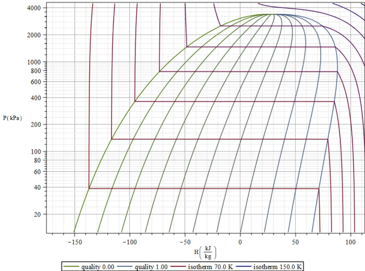
Thermodynamic cycles can be visualized by placing plot objects on these charts. For example, see the [Refrigeration Cycle](#) application.
