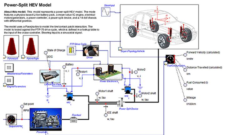
**Figure 4.** Power-split hybrid-electric vehicle model.
