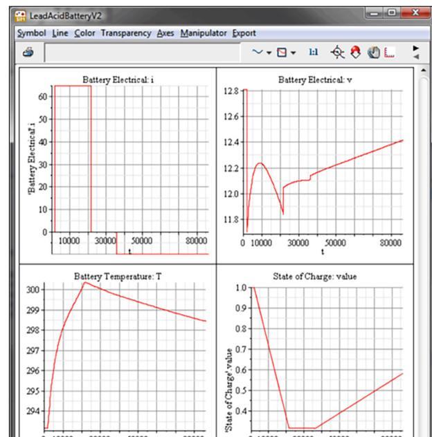
**Figure 3.** The output of a MapleSim simulation of the dynamic response of the battery model. The battery current is shown in the top left plot. First, 65 A is drawn from the battery, the battery rests, then is recharged with 10 A. The dynamic response of the voltage (top right), temperature (bottom left) and state of charge (bottom right) are shown.
