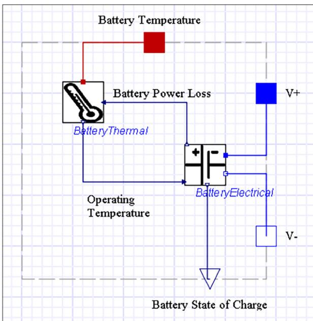
**Figure 2.** The thermal and electrical characteristics of the battery are easily separated and connected in MapleSim.
