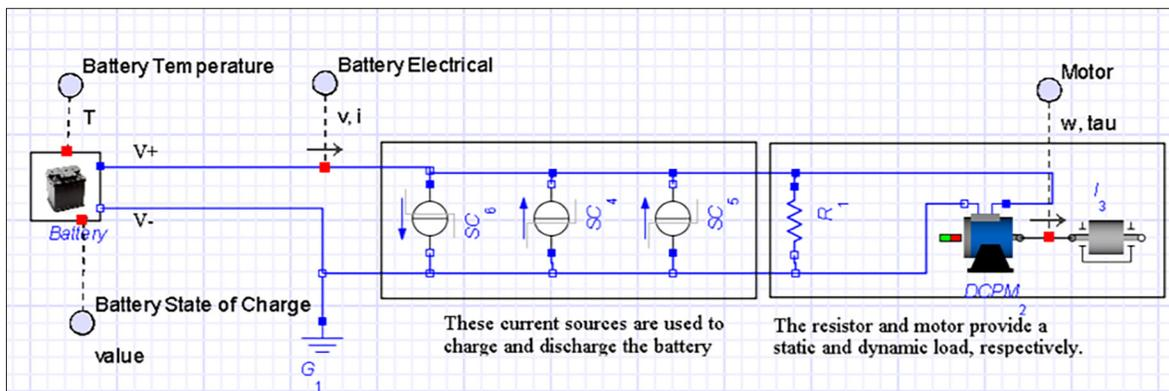
Figure 1. The battery model connected to a variety of loads.
